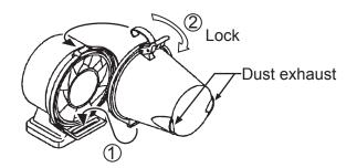
Figure 23. Latching Dust Pot
